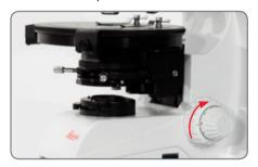
2. Adjust the condenser mount to its lowest position using the condenser focus knob on the left-hand side of the substage.
